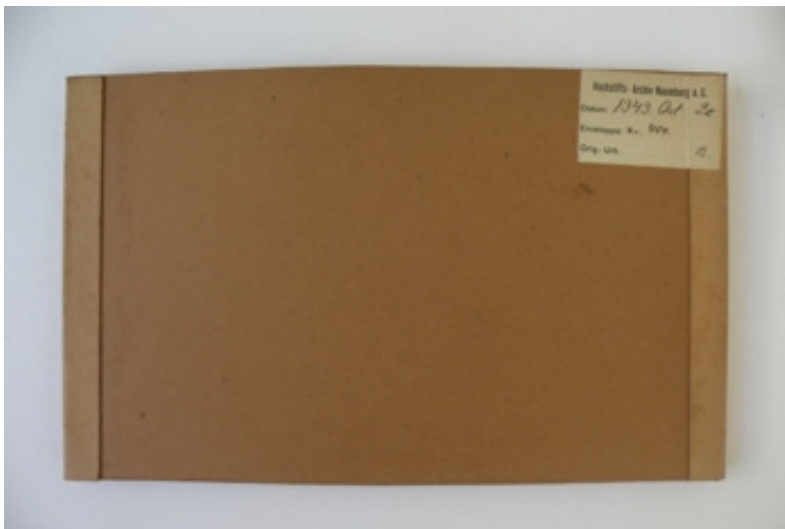
Foto 14: Schubert aus holzschliffhaltigem Material, Format H 22 x B 34 cm (C. Hanke)
